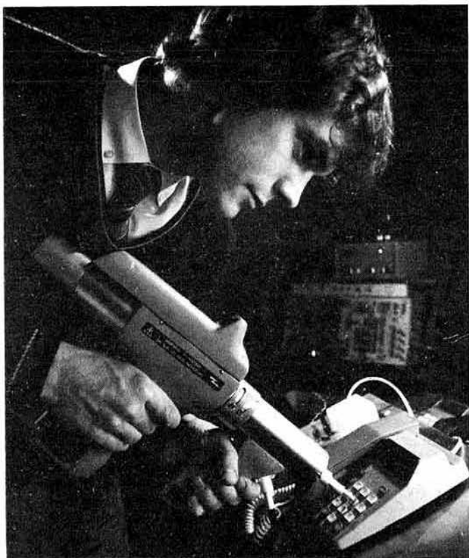
This is not an irate amateur attacking a Sceptre 100 telephone as a result of rfi, but a BTR engineer subjecting it to a static shock of up to 10,000V to ensure that the memory store is not disrupted by static. It also shows up any susceptibility to rfi and resistance to lightning discharges. But did BT carry out such tests before putting their electronic telephones into service?
