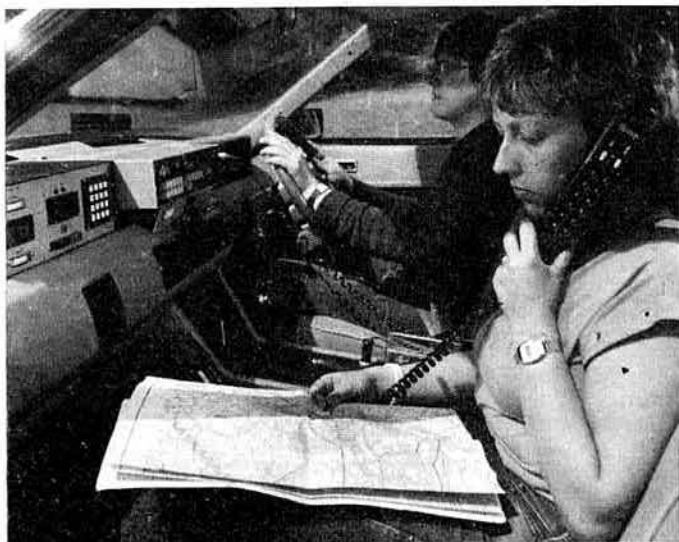
Field trials of the British Telecom/Securicor 900MHz cellular mobile radio system due to be in operation in parts of the UK next year, linking vehicles with the public switched telephone network. In urban areas cells may be only 2km in diameter, in rural areas up to 30km. Cell transmitters are switched by computer-controlled exchanges, automatically transferring the radio links from one cell to the next. But one notes that this photograph shows the mobile telephone being used by a passenger—a lot safer than when used by a speeding driver!
