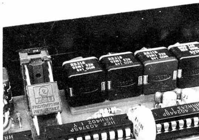
Photo 3. Details of display and potentiometer mountings
